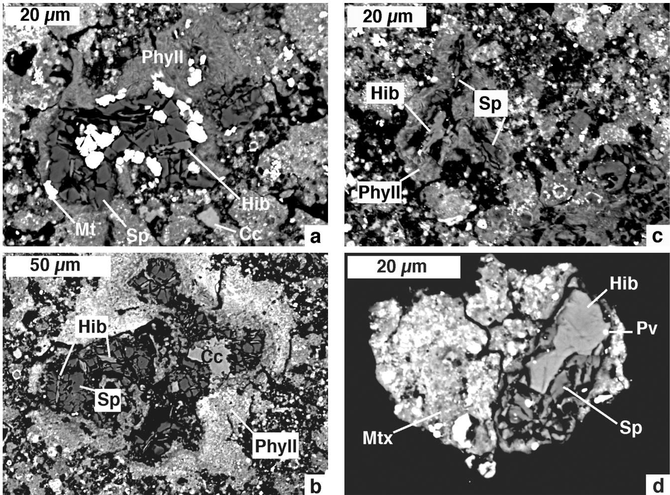
Fig. 1. Backscattered electron images of hibonite-bearing inclusions in Tagish Lake: a) CA2-15; b) CA4-21; c) PB3-27; d) TLDF32. (a)–(c) are in situ and (d) is from the dense fraction. The void spaces and epoxy are black. Cc = calcite; Hib = hibonite; Mt = magnetite; Mtx = matrix; Phyll = phyllosilicate; Pv = perovskite; Sp = spinel.
