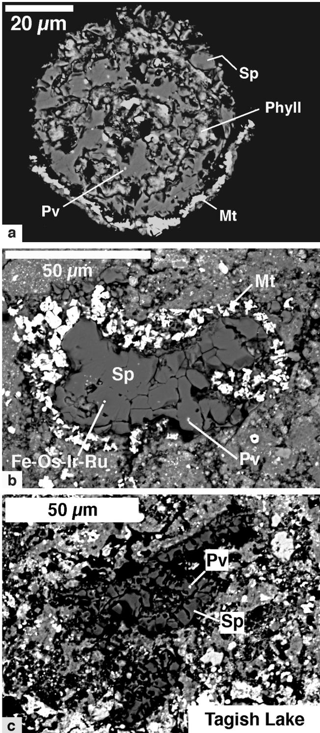
Fig. 2. Backscattered electron images of spinel-rich inclusions in Tagish Lake. Note the fine-grained perovskite enclosed in spinel in all samples: a) a spinel-rich spherule, TL4–29. Note the spherical shape; b) a compact spinel-rich inclusion, CA3–13; c) a fluffy spinel aggregate, CA6–65.
