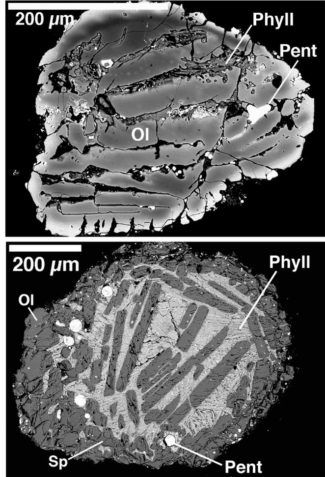
Fig. 3. Backscattered electron images of barred olivine chondrules from Tagish Lake. Note the deformation of the chondrules and complete conversion of mesostasis to phyllosilicate. Ol = olivine; Pent = pentlandite; Phyll = phyllosilicate; Sp = spinel.
