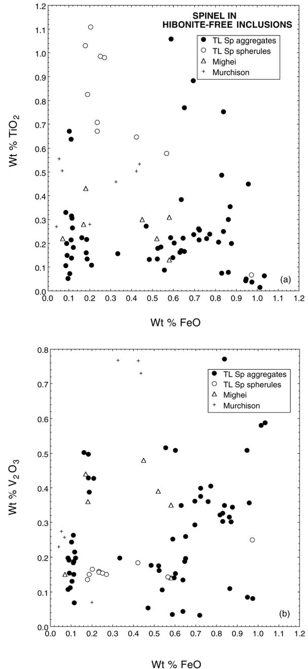
Fig. 8. Compositions of spinel in hibonite-free, spinel-rich inclusions. The range of FeO contents extends to higher values in Tagish Lake spinel than in spinel from Murchison or Mighei. Mighei data are from MacPherson and Davis (1994): a)  $\text{TiO}_2$  versus FeO; b)  $\text{V}_2\text{O}_3$  versus FeO.
