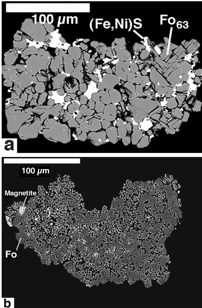
Fig. 4. Backscattered electron images of olivine-rich objects in Tagish Lake. Both are mounted in epoxy: a) a polycrystalline olivine inclusion, TL2–19. Note the irregular shape and lack of mesostasis between grains; b) a forsterite aggregate, TL3–4. Note the porous texture and uniform composition of olivine grains. Fo = forsterite.
