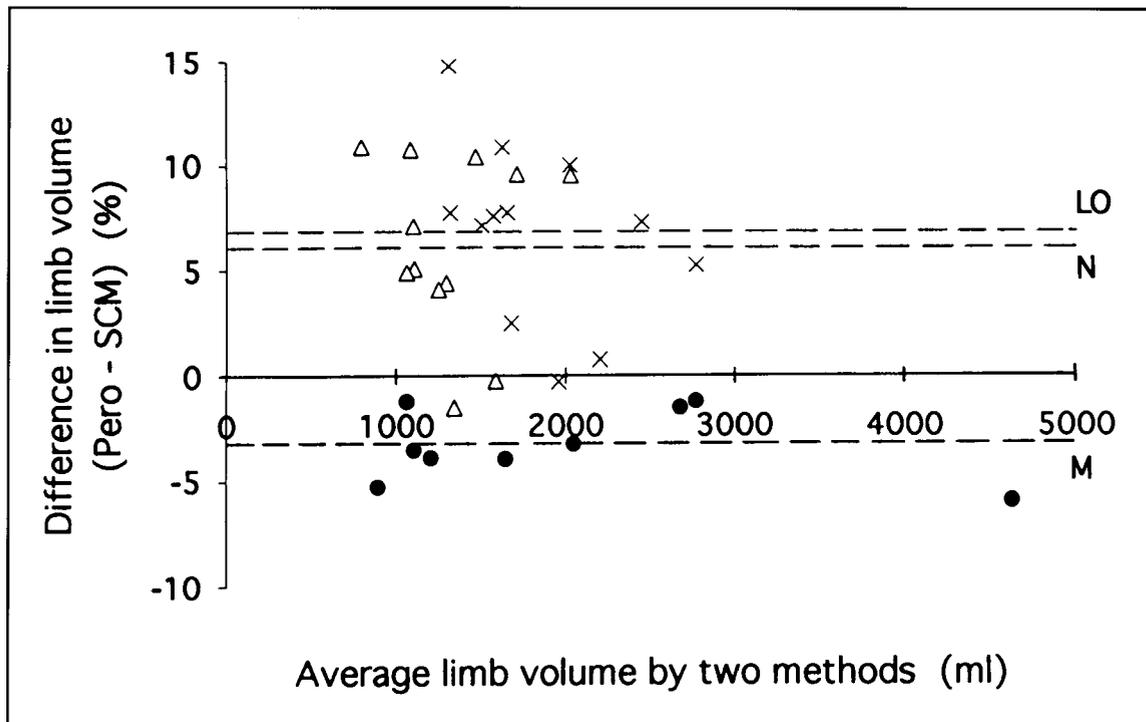
Fig. 3. Differences between the Perometer (Pero) and the sequential circumference method using a tape measure (SCM, tape/frustum method), in the measurement of normal (N, open triangles), lymphoedematous (LO, crosses) and mannequin (M, closed circles) limbs, plotted against the average volume of the two methods (Bland-Altman plot). Dashed lines - mean difference (from 20, with permission).
