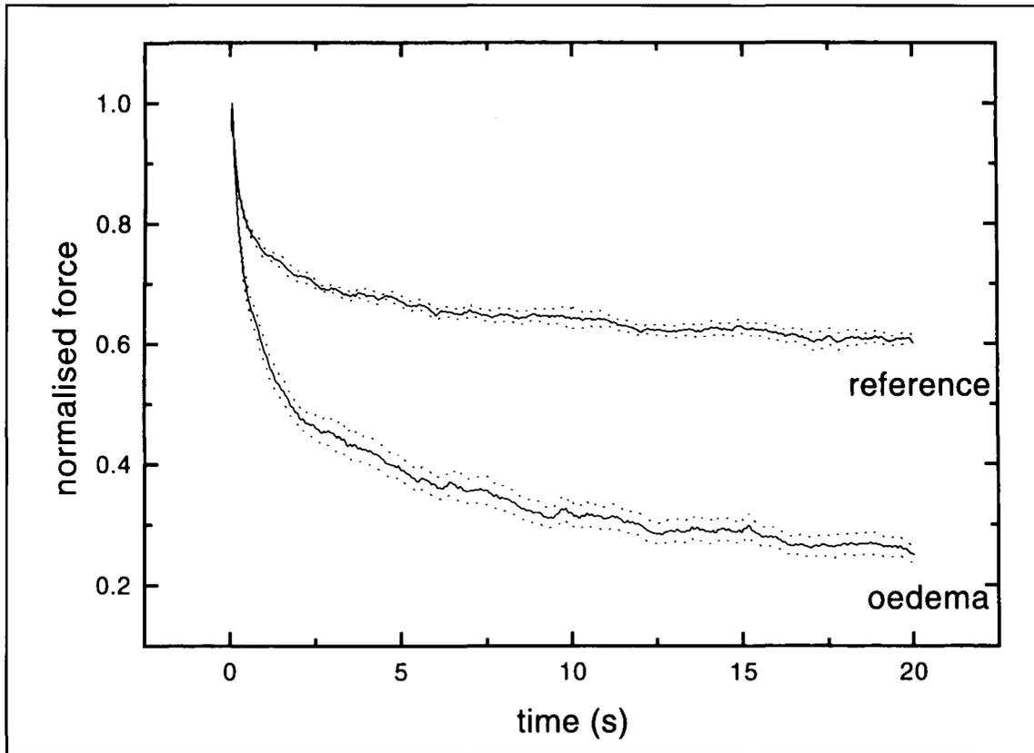
Fig. 4. Declining impression force curves from oedematous and the opposite, normal (reference) arms obtained using the instantaneous step impression method. Solid lines - mean, dotted lines - s.e.m.,  $n = 7$  (from ref. 27, with permission).
