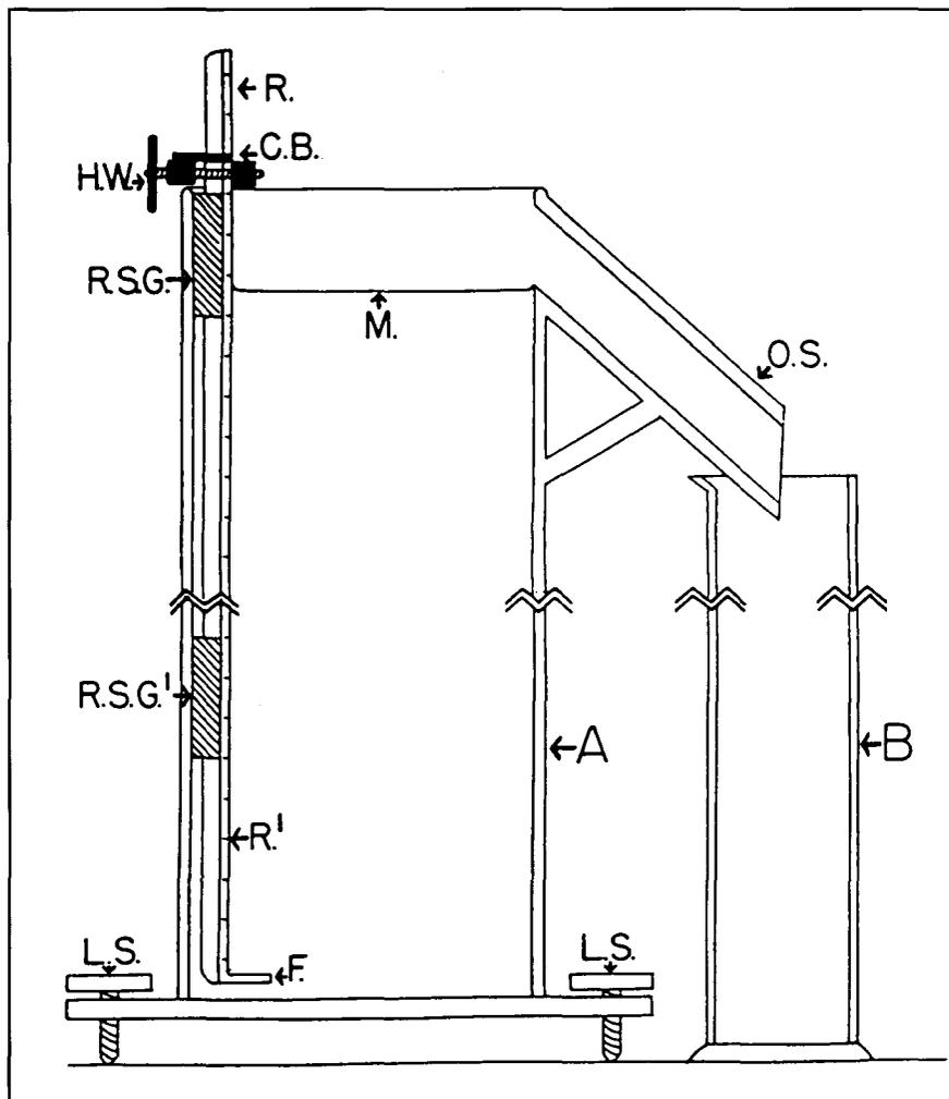
Fig. 1. Sectional diagram of water-displacement apparatus to measure limb volume (from ref. 7, with permission). The tank (A) is cylindrical, made from 1/4 inch Perspex, the base being 1/2 inch thick; B - graduated collecting cylinder; OS - overflow spout; LS - leveling screws; R - metal rule (slides up and down in housing, R.S.G. attached to wall of tank); F - adjustable shelf; HW - hand wheel (fixes rule and shelf in position); CB - cursor block; M - meniscus of water.
