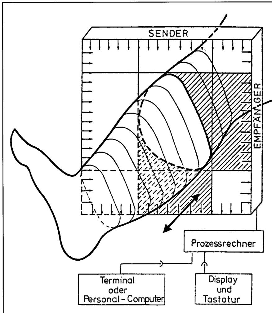
Fig. 2. Diagram of operation of the Perometer (reproduced with permission from Professor J-U Fischbach).
