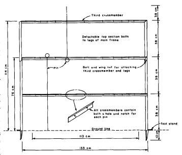
Fig. 1. Diagram of the point frame showing third crossmember and pin spacings.
