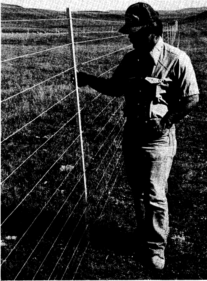
Fig. 1. A 12-wire, 168-cm high electric fence tested in North Dakota. This fence effectively excluded coyotes.
