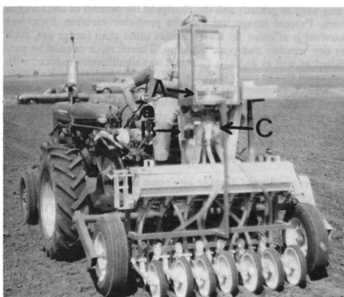
Fig. 2. Rear view of the grass plot drill in operation showing cone (A), electric motor for the spinner (B) and the divider (C).
