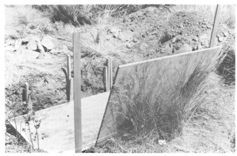
Fig. 2. Display board placed against the prepared surface after the thick solution of cellulose acetate has been applied.
