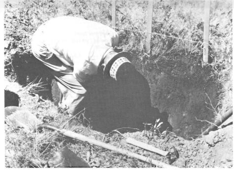
Fig. 1. Shows area marked off and soil face being smoothed down ready to apply the thick solution of cellulose acetate.
