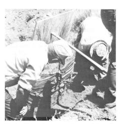
Fig. 3. Tying the range soil monolith to the display board before removing from the pit.
