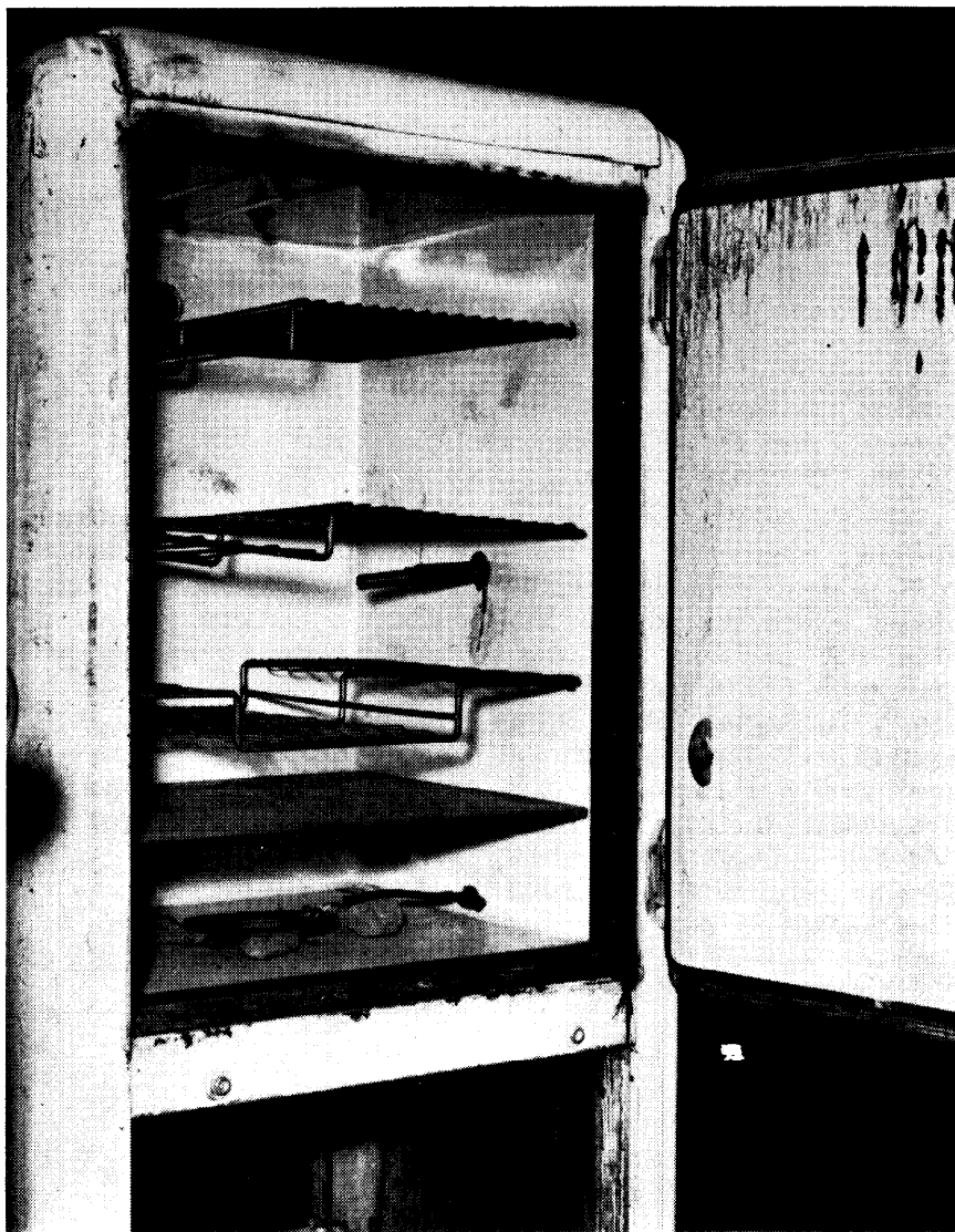
FIGURE 1. The drying oven interior showing coil, steel plate, thermostat and racks.
