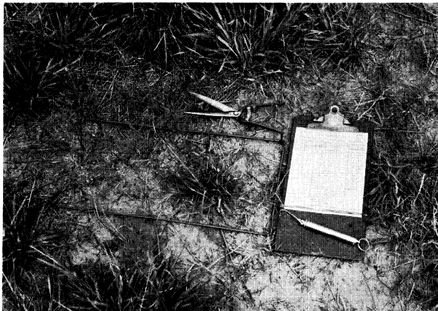
FIGURE 3. Primary equipment (shears, micro-plot quadrat, field forms, and gram scales) needed to inventory forage by the micro-unit method.
