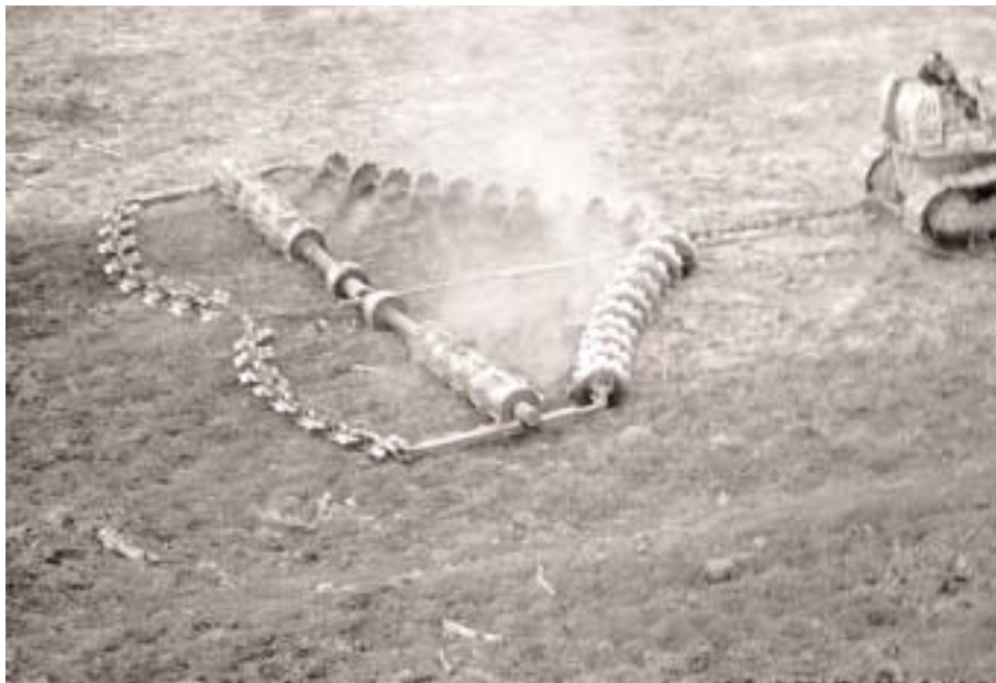
Fig. 1. Chain diker attached to rear of the disk chain was designed to form basins in soil tilled by the disk chain during seedbed preparation on land littered with brush debris. The implement is called a disk-chain-diker (Wiedemann and Cross 1994).
