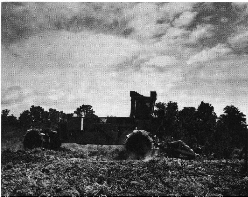
FIG. 6. Tree crusher in action—control and cleanup is accomplished in one operation. Readily available fuel wood is a side benefit of this technique.
