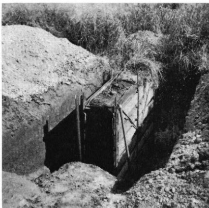
FIG. 2. Soil-block encased in "steel frame" ready for removal to laboratory for washing. This block weighed in excess of 3400 pounds.
