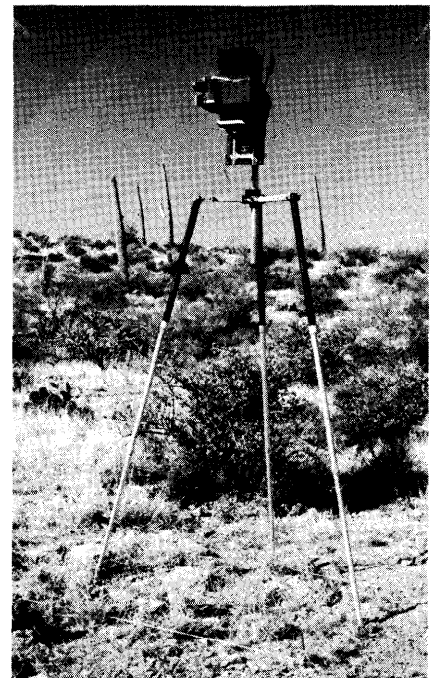
FIG. 1. Crown-Graphic camera with Polaroid back mounted on a modified tripod ready to take photograph.
