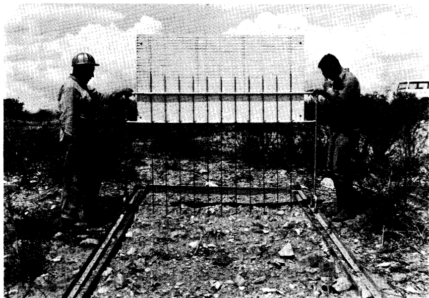
FIG. 1. Reliefmeter in place on a cleared, pitted, and seeded plot. Measurement being made prior to onset of summer rainy season 1964.
