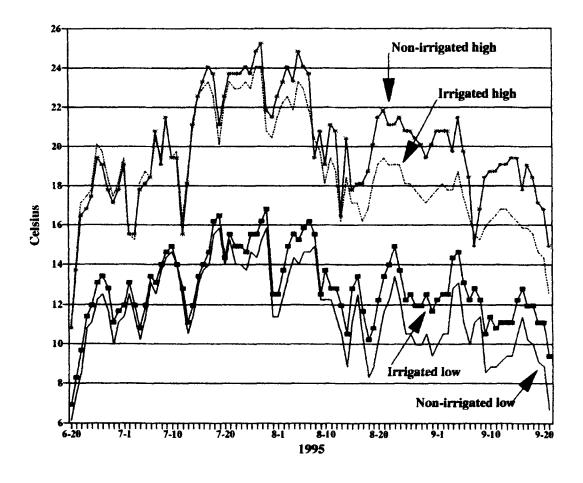
Fig. 2. Daily maximum and minimum water temperatures in stream reaches contained within adjacent non-irrigated and irrigated meadows.
