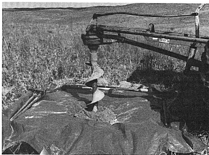
Fig. 1. Tractor-mounted auger used to drill holes to place containers in the ground. A tarp was used to collect soil for placement in containers and to minimize disturbance to the area.
