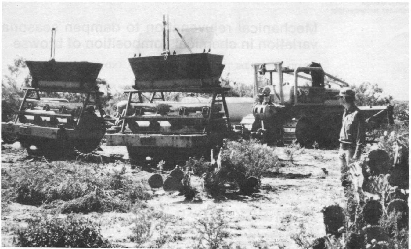
Fig. 1. Two roller choppers pulled in tandem by a crawler tractor to remove top growth of shrubs in southern Texas.
