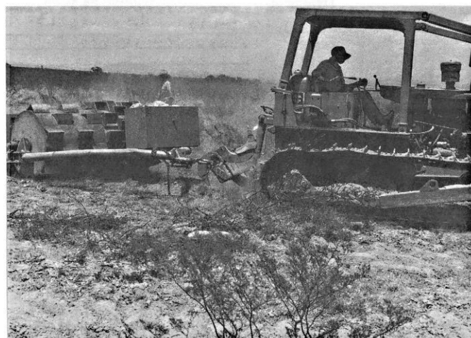
Fig. 2. Land imprinter pulled by track tractor. Note iron box filled with rocks mounted on frame and V-pitter geometry of left capsule and pit-digger geometry of right capsule.
