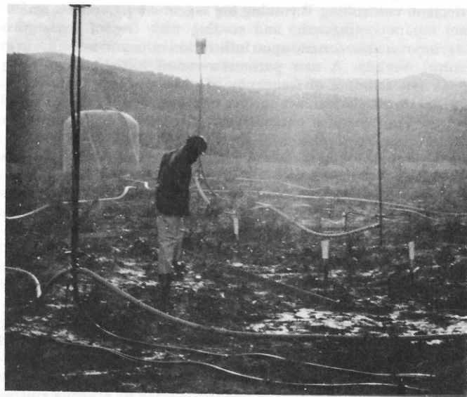
Fig. 1. Rainfall simulator sprinkling water on a plowed and seeded plot.
