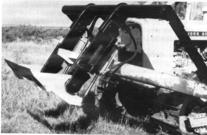
Fig. 2. Unique hydraulic attachment increases tree size uprooting capacity of low-energy grubber. Blade rotation of 70° results from extending the hydraulic cylinders and action aids in tearing roots loose and stump uprooting.
