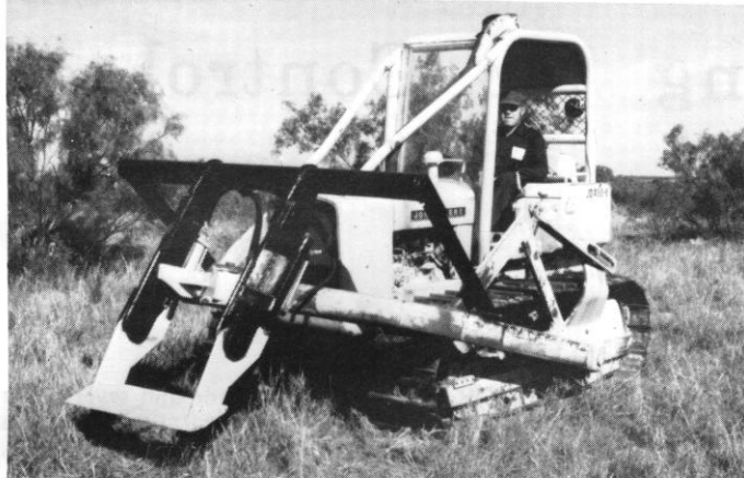
Fig. 1. Low-energy grubber developed by Texas Agricultural Experiment Station engineers to control small trees infesting rangeland. The small, 48.5-kW (65-hp), crawler tractor was adapted for grubbing by attaching special U-shaped blade to the front-mounted C-frame.
