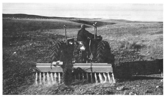
Fig. 2. Spreading sodium carbonate with calibrated fertilizer spreader.
