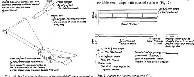
Fig. 1. Pictorial sketch of certain elements of rangeland drill, showing position of one set of modification parts for lifting drill-arm assembly.
