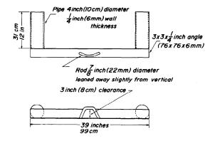
Fig. 3. Wheel chocks for securing rangeland drill.
