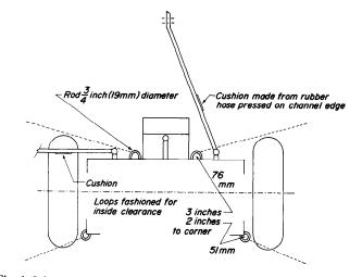
Fig. 4. Schematic sketch of rangeland drill, showing tie-down loops positioned to secure implement on trailer with maximum front-to-back stability during transport. Drill rests sideways on trailer.
