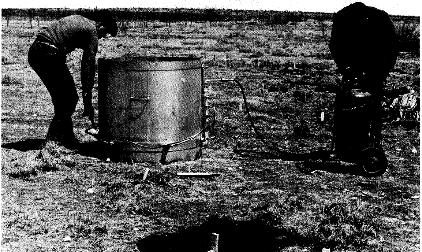
Fig. 1. A specially designed propane burner was constructed from stainless steel to burn the plants individually. Heat treatments were controlled by pressure of propane gas at the nozzle in relation to time as shown in Figure 2.
