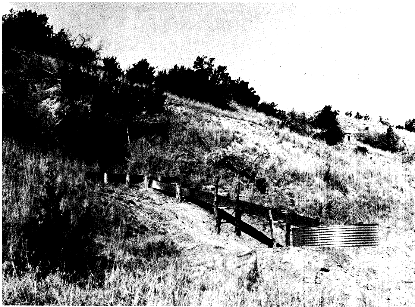
Fig. 1. A metal dyke with trough and collection tank were installed at the base of each watershed.
