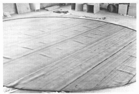
Fig. 2. Thirty-foot diameter floating cover fabricated from 48-inch wide, low-density, closed cell rubber sheet stock.
