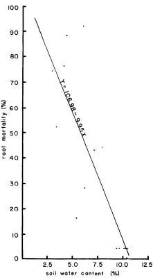
Fig. 2. Relationship of average surface (0-6 inches) soil water content to average mesquite mortality from Tordon 225 Mixture applied in 1970. Average is based on 25 trees on 15 sites (except one, which is the average of 23 trees). Mortality was determined following the second growing season after herbicide application.
