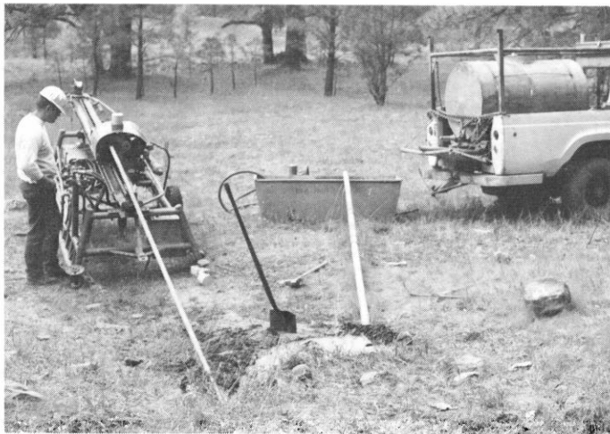
Fig. 2. Horizontal well drilling equipment should be as light and portable as practical for use in rough range country. Note that water is recirculated through a rotary wet-boring drill stem. The heart of the rig is a pipe chuck which turns at about 100 rpm and is powered by a 10 hp gas engine.
