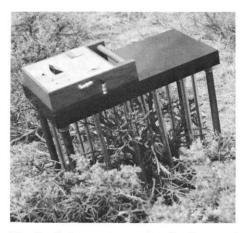
Fig. 2. Herbage meter on plot after leaves and current annual growth of shrub stems were removed.
