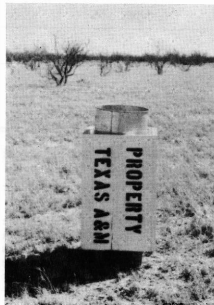
Fig. 1. The assembled rain-snow gauge in service.
