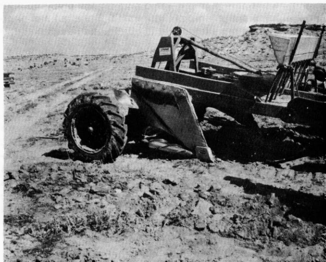
FIG. 1. The soil ripper, pulled behind a crawler tractor, effectively breaks up soil to a depth of about 28 inches.
