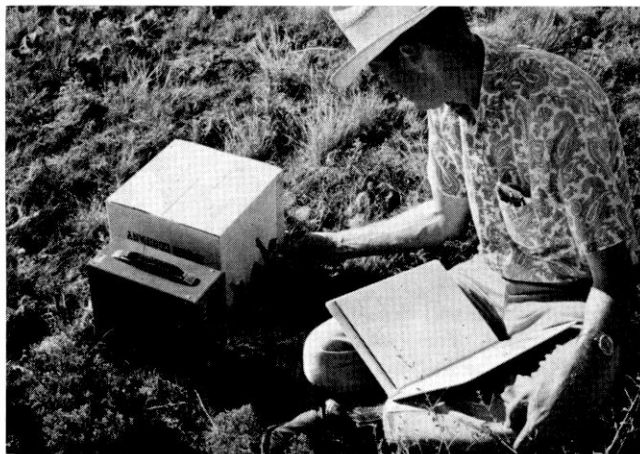
FIG. 3. A view showing the relative positions of the G-M tube and the box which holds the beta-emitting source.
