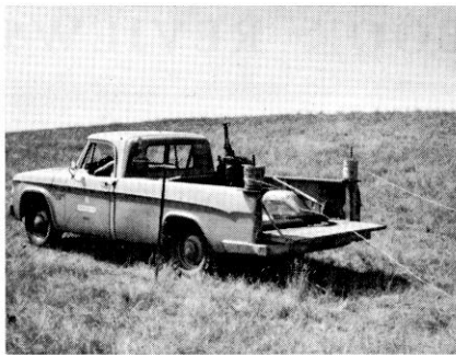
FIG. 2. With the vertical dispenser, friction keeps some tension on the wire, and prevents spin-caused entanglements.
