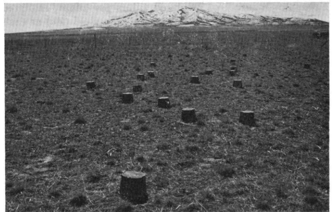
FIG. 1. Inverted plastic pots being used to stimulate etiolated growth of crested wheatgrass as a field method to assess organic reserves.
