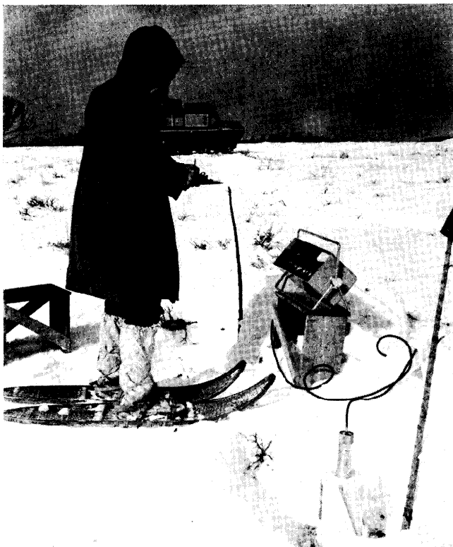
Fig. 1. Winter soil moisture measurements with neutron-probe equipment.
