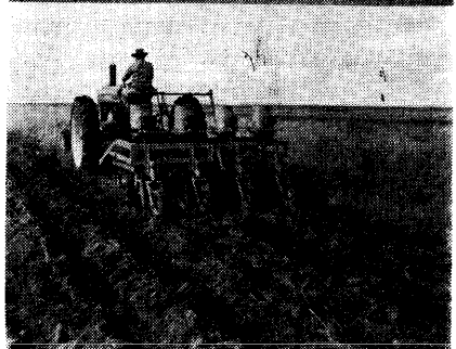
FIGURE 2. Top—The double-disc depth-band drill on a prepared seedbed. Bottom—The lister-type grass planter on a direct-seeding plot.
