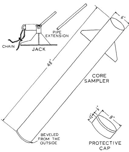
FIGURE 1. Sketch showing the construction of a simple core sampling device, its protective cap, and the jack for removal of cores from the soil.
