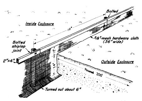
FIGURE 2. Construction detail of exclosure fence.
