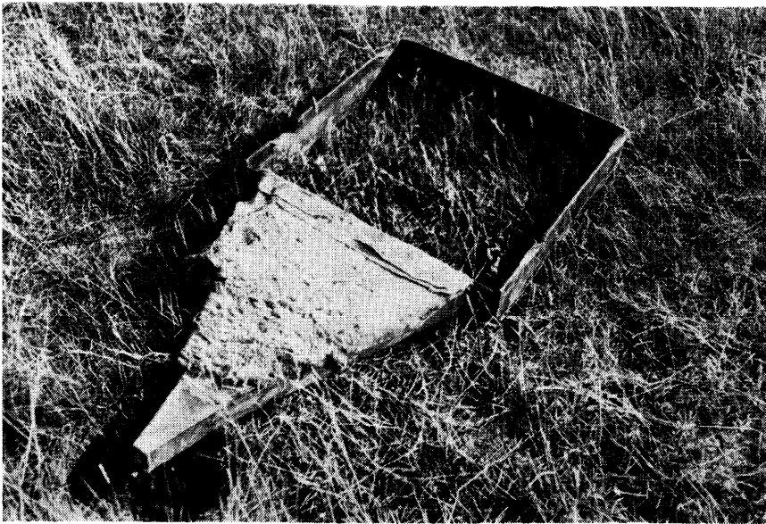
FIGURE 2. Two by two foot square plot enclosure with runoff spout attached as used in this study. The burlap on the spout is to absorb simulated rainfall to prevent splash into the plot.
