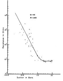
FIGURE 1. Calibration curve for Bouyoucos resin impregnated gypsum blocks.
