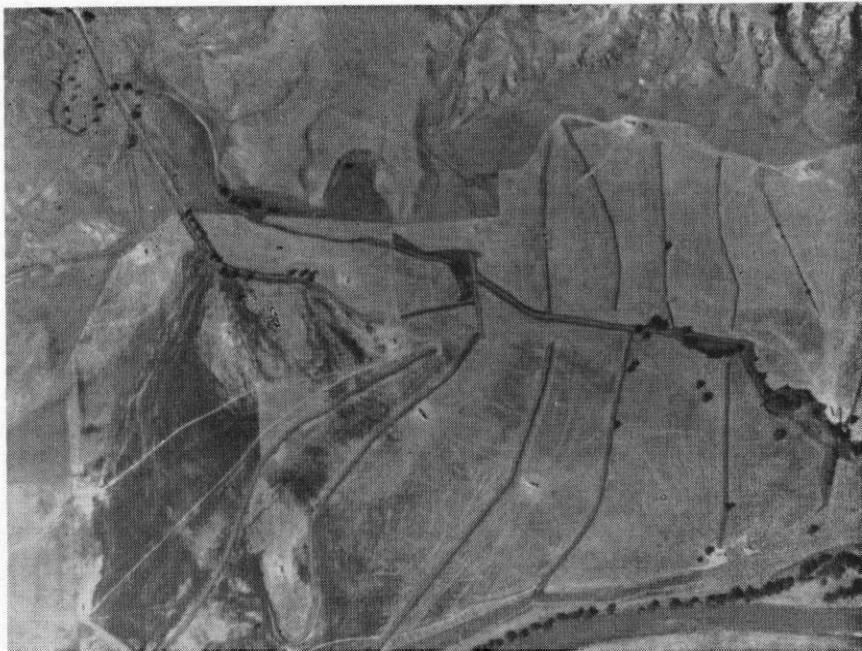
Water is impounded and spread by means of dikes from Haydraw, a 40,000 acre drainage. Excess water leaves the flat through a natural channel to the right, prevented from flowing into the river (lower right) by a dike along the bank.
