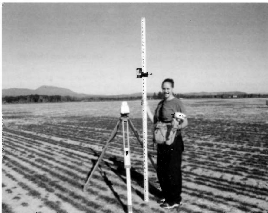
Fig. 1. Equipment used to generate highly accurate digital elevation models include a laser level and a sliding laser receiver attached to a leveling rod. In the horizontal mode, the laser level self levels via a wire-hung, air-damped compensator. The Pro Shot® L4 (Laser Reference, Inc.) laser level we used has a working radius of 230 m, with a leveling accuracy of 1.6 mm per 30 m.
