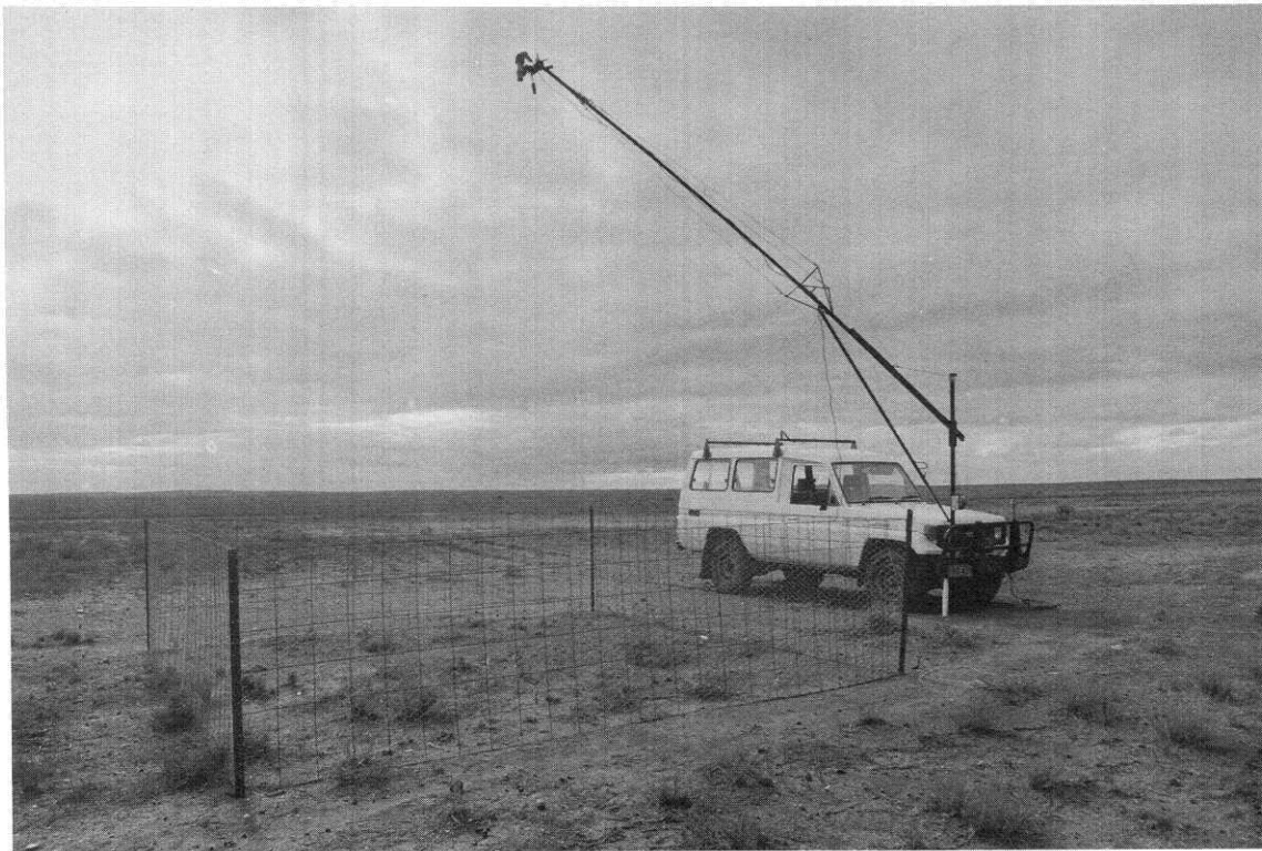
Fig. 3. Photograph of mobile system used to map large plots in western New South Wales.
