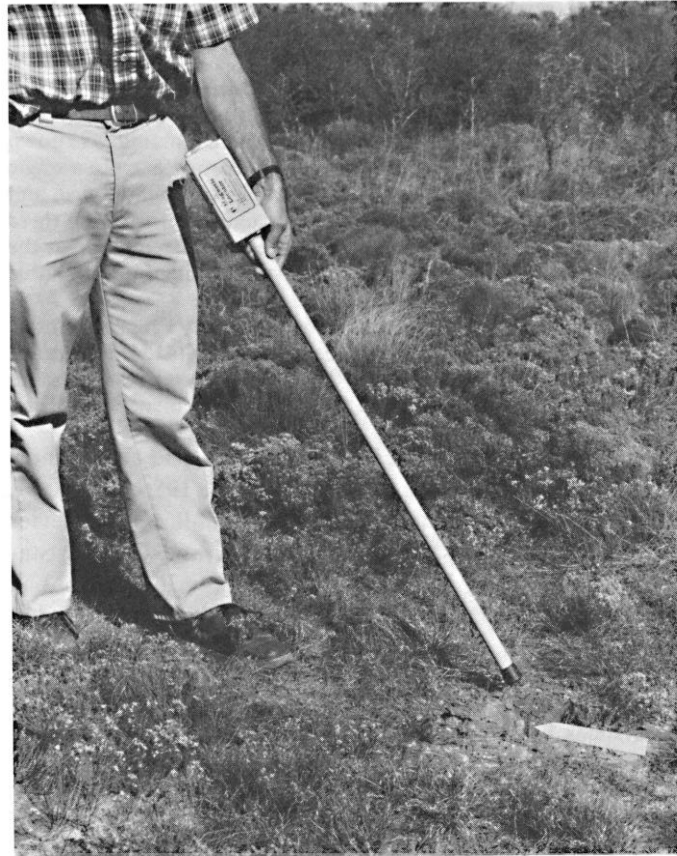
Fig. 1. Metal detector locating steel stake (arrow) which would be below the soil surface.
