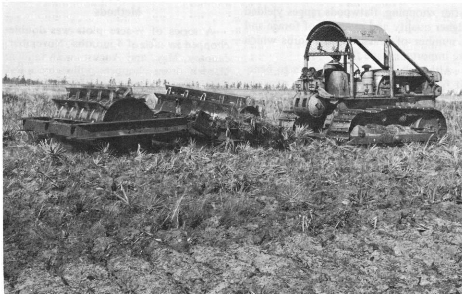
Fig. 2. Drum choppers pulled in tandem give effective mechanical control of unwanted vegetation.
