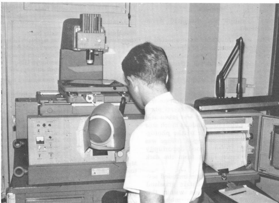
Fig. 1. Microdensitometer (left) with a strip chart recorder attached (right).
