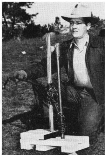
FIGURE 1. Soil tube puller in operation, showing the soil tube and arrangement of bumper jack, chain and platform. The black part of the platform is 1½-inch angle iron; the remainder is constructed of wood.
