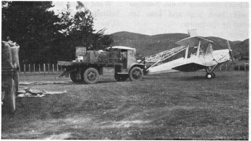
FIGURE 2. Loading a light plane for aerial topdressing. Rapid mechanical loading devices minimize the time planes are on the ground. (Courtesy Grasslands Div., N. Z. Dept. Sci. and Ind. Res.)
