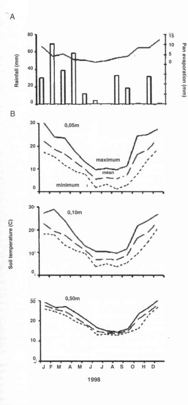
Fig. 1. A) Daily rainfall (mm; vertical bars) and PAN evaporation (mm; solid line), and B) Absolute maximum and minimum, and mean monthly soil temperatures measured at 0900 hours at 0.05, 0.10, and 0.50 m soil depth during 1998 at a meteorological station located at the study site.
